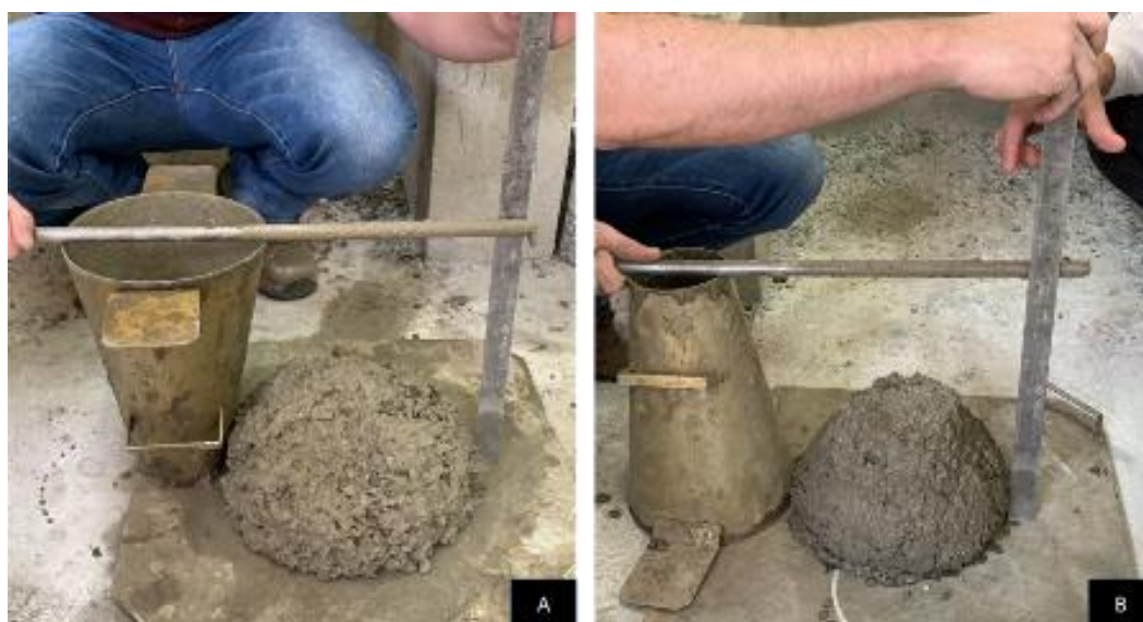
Figura 14 - (A) Slump Test CP-25; (B) Slump Test CR
