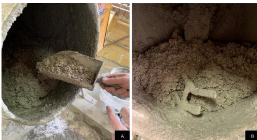
Figura 13 - (A) Concreto fresco CR; (B) Concreto fresco CP-50
