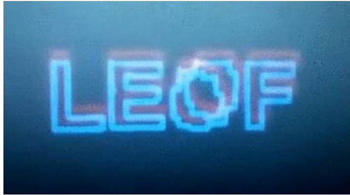
Figure 42 - LEOF Acronym produced by our micromachining setup in a gold thin film
